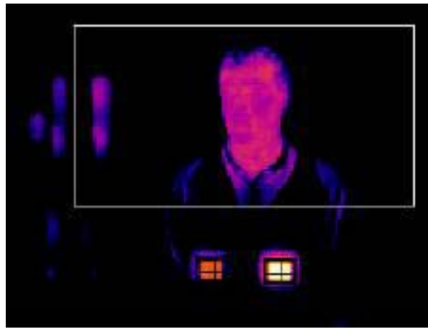
Figure 7 - Typical Output by Type Three Thermal Scanner. Note the two thermal reference sources shown at the bottom of the figure (Wang, 2004).
